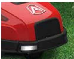
Bumper & Active Mechanical Obstacle Sensor
