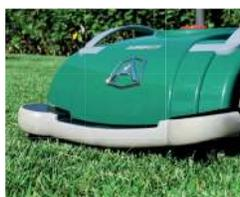
Bumper With Mechanical Obstacle Sensor
